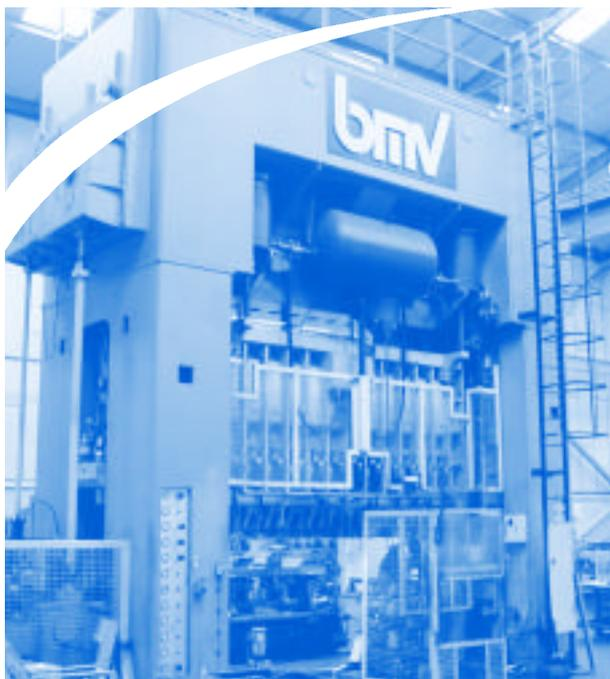
800-ton transfer press machine for door hinge manufacture.
