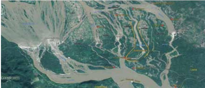
The powerhouse of the Project will be located at the southern end of the Sahong channel, one of seven major channels of the Mekong River in the Siphandone (Four Thousand Islands) area that flow over the geological feature called the "Great Fault Line". The Project would utilise on average only about 15% of the total Mekong flow. This, coupled with the existing channel configuration, that provides natural spillways
